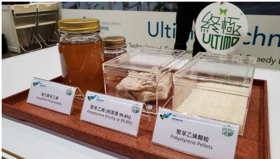
Recycled PS material generated from EPS wastes using Ultimo Technology™
